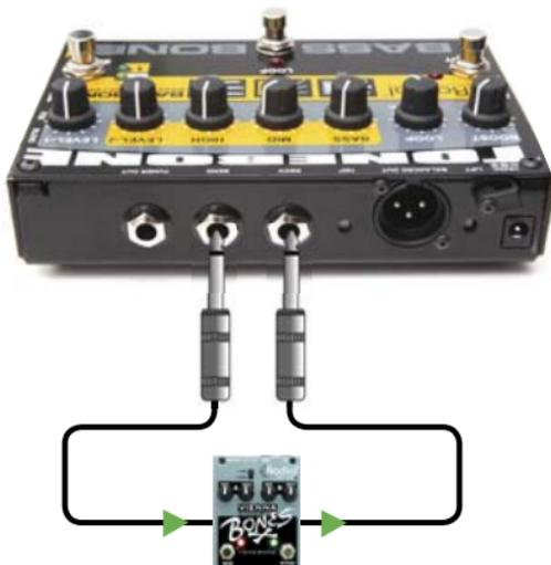
Depress the LOOP footswitch to turn the function on, the LED indicator will illuminate. *Note: If there are no pedals connected to the SEND and RECV jacks the LOOP footswitch will have no effect on the sound. You cannot accidentally mute your sound because there are no pedals connected.*
