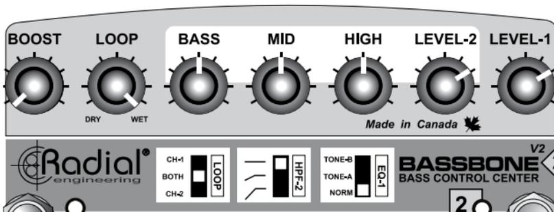
Some of the Bassbone functions are controlled by 'set & forget' switches on the side panels. These switches are recessed to prevent accidental use and can be accessed with a small screwdriver when needed. Ensure all five of these switches are set to their outward positions to start with.
