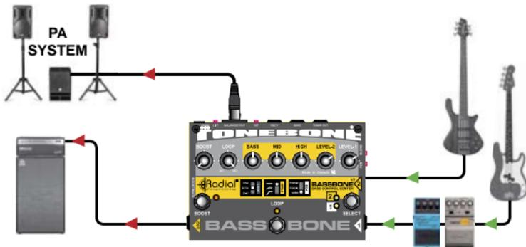
You could also introduce a series of pedals between the Bassbone's 1/4" output and your amp. This way the pedals can be heard through your amp but the effects will not be sent to the PA system if using the balanced XLR output.
