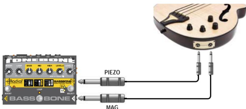
Some basses use a 'stereo' jack to output both pickup signals. If your bass uses one stereo TRS  $\frac{1}{4}$ " jack you can use an 'insert' type cable where the signal is sent to separate  $\frac{1}{4}$ " plugs. Because channel-2 is optimized for acoustic piezo pickups, you will want to ensure the the piezo pickup is connected to channel-2.
