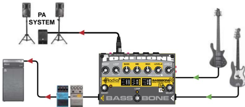
To take things one step further, the Bassbone is equipped with a unique effects loop designed specially for bass. The effects loop lets you insert pedals by depressing a footswitch and mix the effects with the original bass signal to preserve the fundamental tone of your bass. You can also assign the effects loop to channel-1, channel-2 or both, giving you absolute freedom. Connected this way, the pedals will be heard through your amp and in the PA system.
