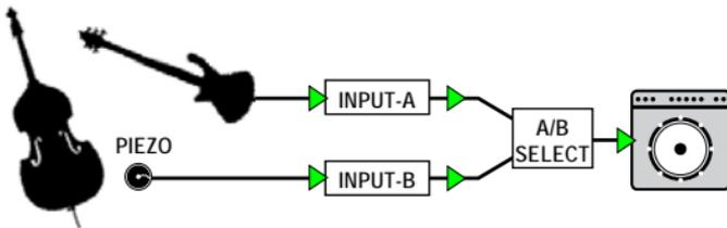
**Mixing two pickups:** Players that use acoustic/electric basses with two pickup systems can employ the Bassbone's unique BLEND function. This turns both channels on and lets you mix the sound of both pickups.
