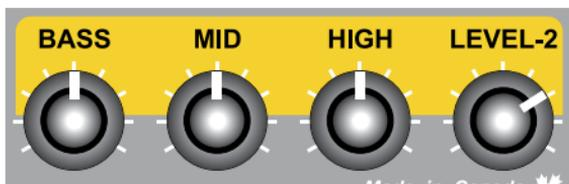
The three-band EQ can dramatically increase or decrease the amount of gain depending on the settings. For instance, rolling off low end with the EQ will reduce the overall gain. Compensate by adjusting the LEVEL-2 gain until it matches channel-1. Once the EQ and level controls are set, you can toggle between channels without adjusting your amplifier's volume or EQ settings.
