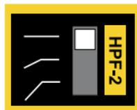
The HPF-2 filter has a flat setting (filter bypassed) and two settings that gently roll off bass. The middle setting rolls off low frequencies below 35Hz and the bottom setting below 60Hz.
