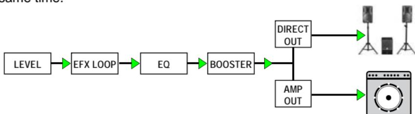
Connect the direct output to the microphone input of a mixing console using standard XLR cable up to 100 meters (300'). The XLR male connector is wired to AES standards with pin-1 ground, pin-2 hot (+) and pin-3 cold (-).
