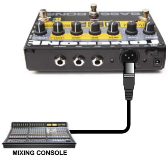
The direct output is equipped with a ground lift and a polarity reverse. The recessed ground LIFT switch helps eliminate hum and buzz caused by ground loops. If you hear noise try pushing the ground LIFT switch inward.
