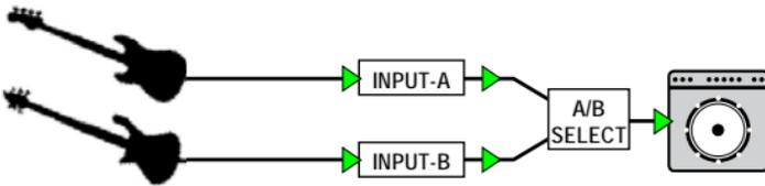
**3. Switching between upright bass and electric bass:** The Bassbone is equipped with a special PZB booster circuit that allows a passive piezo transducer to connect directly to INPUT-2. This lets you quickly transition from an electric bass to a piezo equipped upright bass.
