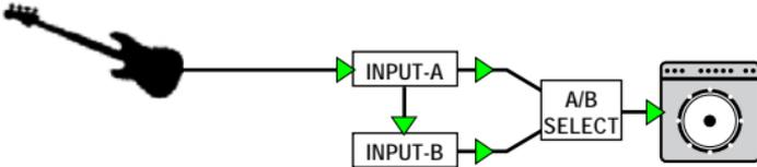
**2. Using with two basses:** Connecting a second instrument to the INPUT-B jack turns the Bassbone into a two *instrument* preamp. You can toggle between instruments by stomping on the footswitch.
